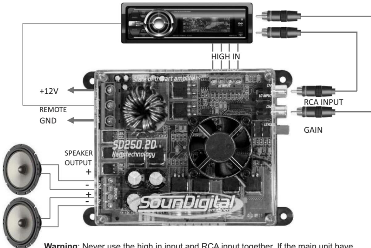
**Warning:** Never use the high in input and RCA input together. If the main unit have RCA output, use only this output, if doesn't have, use the high output.
