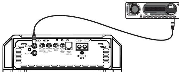
Exemple of two RCA cables connection (mono input).
