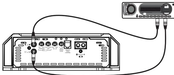
Exemple of one RCA cable connection only and using the RCA output to connect another amplifier.
