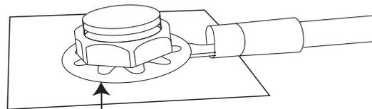
Remove the paint between the terminal and chassis
