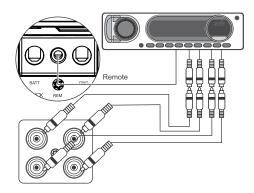
All RCA Inputs must be connected for the 4 channels to work.
