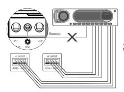
All High signal Inputs must be connected for the 4 channels to work.
