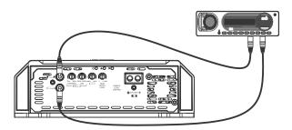
Example of one RCA cable connection only and using the RCA output to connect another amplifier.
