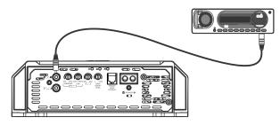
Example of two RCA cables connection (mono input).
