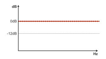
Switch key to "HP" - Set in the variable control between 45Hz and 850Hz ("A") where you want to perform the high pass cut filter;
