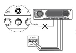
All High signal Inputs must be connected for the 4 channels to work.
