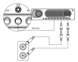
All RCA Inputs must be connected for the channel work.
