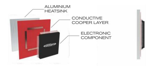
The **DTR**\* is a dynamic thermal recovery system which always maintains a high efficiency of the amplifier by accelerating the thermal exchange of electronic components with the heatsink
