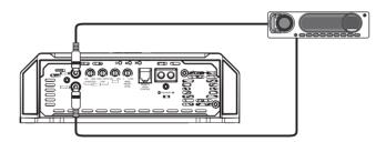
Example of one RCA cable connection only and using the RCA output to connect another amplifier.
