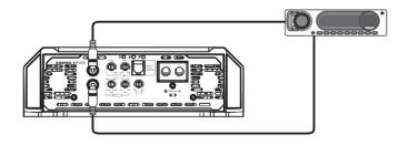
Example of one RCA cable connection only and using the RCA output to connect another amplifier.
