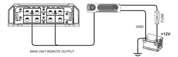
AUDIO INPUT AND OUTPUT CONNECTIONS
