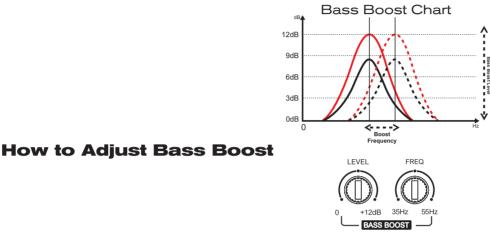
Reproduce your favorite song and set the variable frequency control to the frequency you want boost between 35Hz and 55Hz. Set boost intensity between 0dB and +12dB at the variable control Level.
