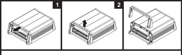
Carefully pull out the top of plastic cover to release the upside latches, as shown in the picture 1.
