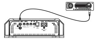
Example of two RCA cables connection (mono input).
