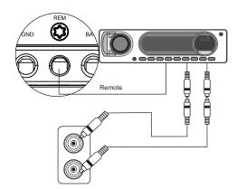
All RCA Inputs must be connected for the 2 channels work, including the Bridge Connection
