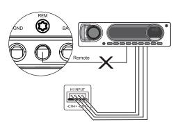
All High Signal Inputs must be connected for the 2 channels work, including the Bridge Connection
