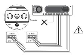
All High level signal inputs must be connected for the all channels to work properly.
