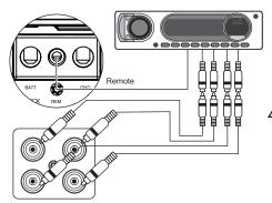
All RCA inputs must be connected for the all channels to work properly.
