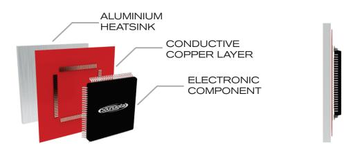
The **DTM**\* is a dynamic thermal recovery system which always maintains a high efficiency of the amplifier by accelerating the thermal exchange of electronic components with the heatsink.
