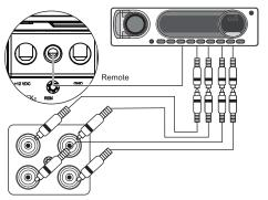
All RCA inputs must be connected for all the channels to work properly.
