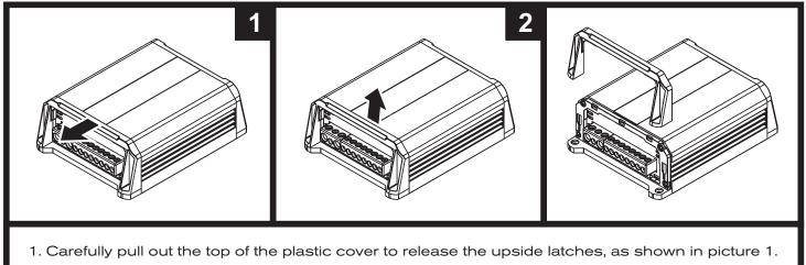
2. Slide up the plastic cover in a continuous movement to remove it.
