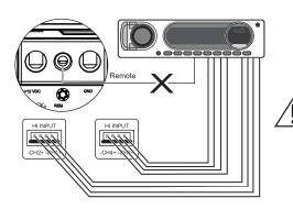
All High level signal Inputs must be connected for all the channels to work properly.
