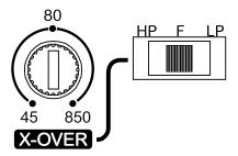
"F" All the frequencies will be reproduced; "LP" Set in the variable control on Low Pass Function; "HP" Set in the variable control on High Pass Function.
