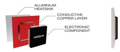
The **DTM**<sup>\*</sup> is a dynamic thermal recovery system which always maintains a high efficiency of the amplifier by accelerating the thermal exchange of electronic components with the heatsink.
