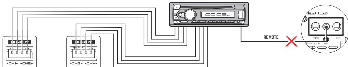
High level input must be used when the main unit does not have RCA outputs.
