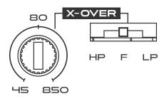
"F" All the frequencies are reproduced; "LP " Set in the variable control on Low Pass Function; "HP " Set in the variable control on High Pass Function.
