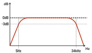
• Change the switch to "HP" position - Set in the variable control between 45Hz and 850Hz ("A") where you want to perform the high pass cut filter;
