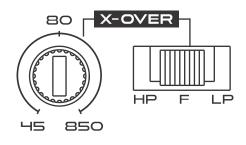
"F" All the frequencies are reproduced; "LP " Set in the variable control on Low Pass Function; "HP " Set in the variable control on High Pass Function.
